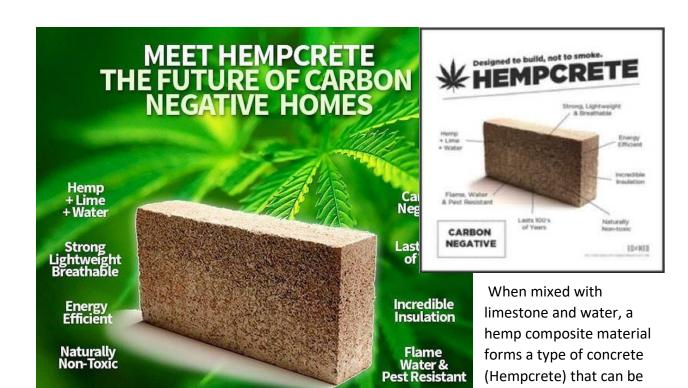
than similar materials (1/9th the weight) and works very well as an insulation material that is airtight, yet breathable, flexible, and repels some vermin. Hemp blocks can be formed into a building material like concrete blocks. They have a high thermal mass capacity that stores energy and releases it gradually. The blocks are resistant to insects, fungi, mold, mildew, fire, rodents, and termites.
